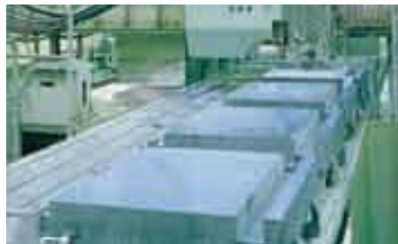
Grinding CMM granite tables on a large grinding machine
